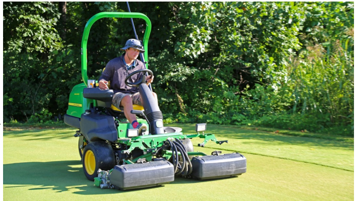
Using a triplex to mow greens can save a significant amount of staff time with no discernable impact on playability.
